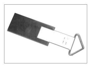
2. Place the test plates with test specimens in the bridges and lightly fix them with the crossbeam and screws.
