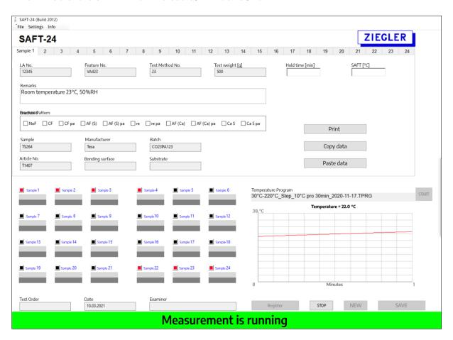
The testing of the samples is carried out using the included SAFT-24 software. The program offers you maximum comfort when processing your data. The clear and intuitively designed user interface convinces by reducing the training to a minimum of time. Within the software, 24 test stations can be edited and checked individually.
